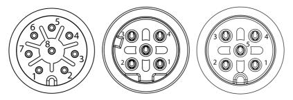
Figure 5: M12 connector pinout, 8-pin A-coded, 4-pin D-coded and 5-pin A-coded.
